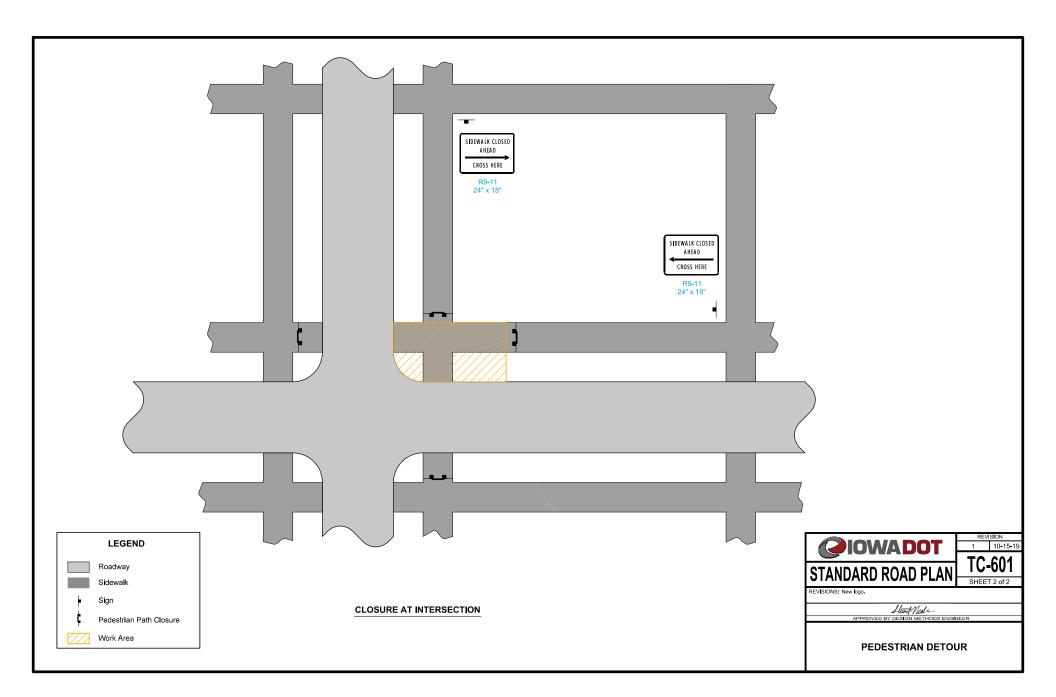
Acceptable materials and construction method for Pedestrian Channelizer will be defined in the contract documents. When Temporary Barrier Rail is specified as the Pedestrian Channelizer, Section 2528 of the Standard Specifications applies. For other types of Pedestrian Channelizers, the length of Pedestrian Channelizer installed will be measured in feet. Payment will be at the contract price per linear foct.
