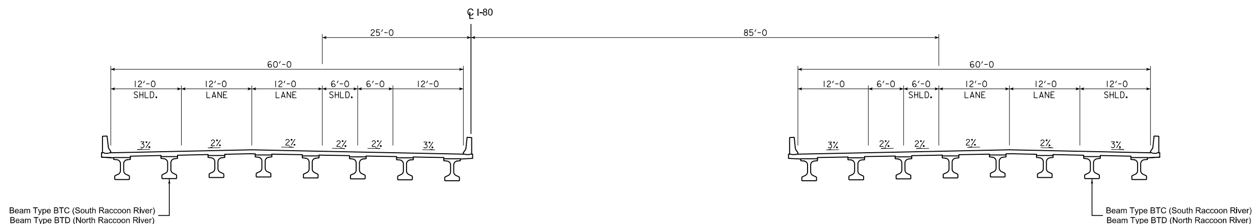
I-80 PROPOSED TYPICAL BRIDGE SECTION
