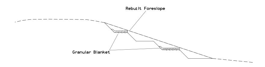
Benches shall extend a minimum of 6 feet into the undisturbed foreslope.
