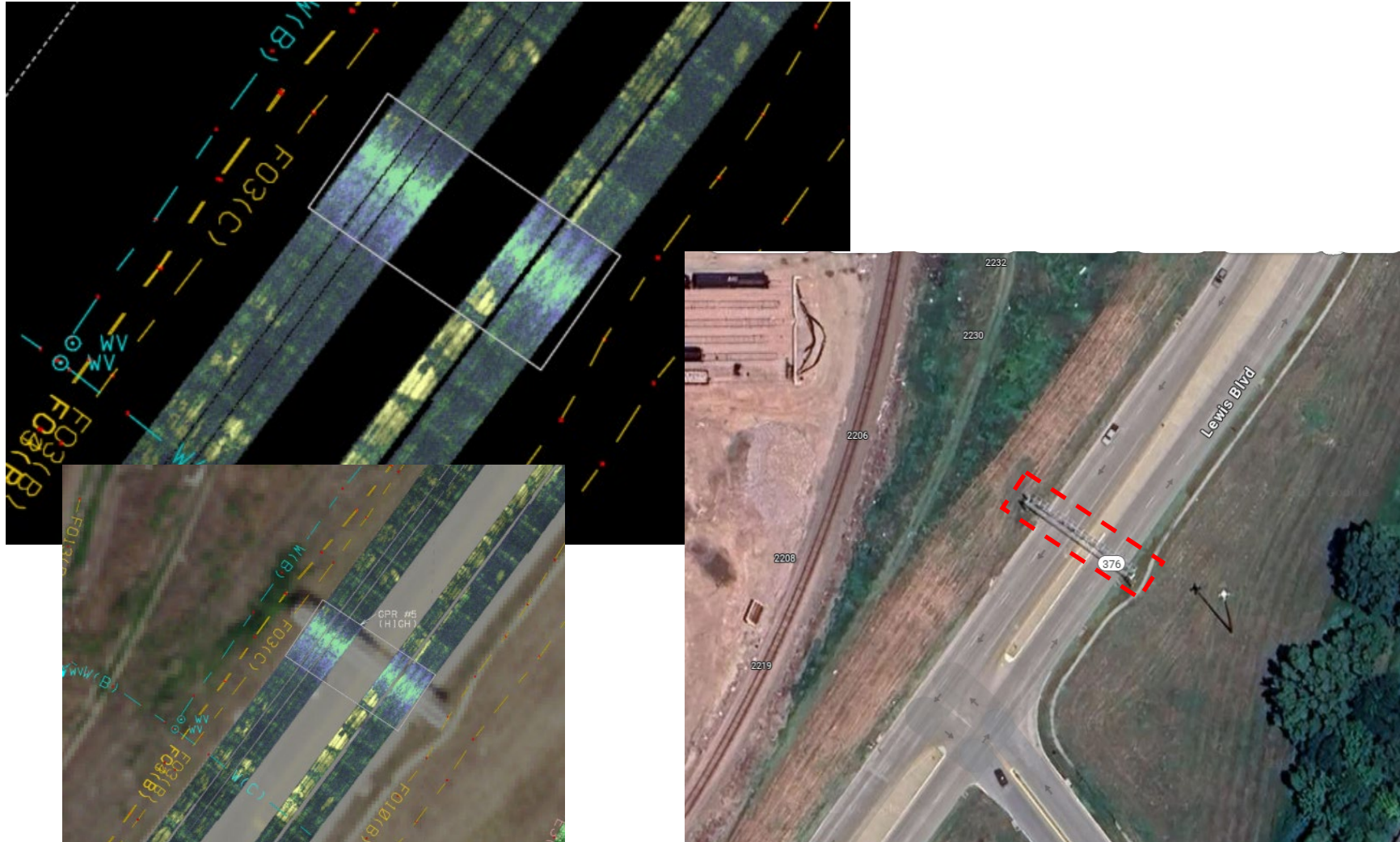
Figure 17. Lewis Boulevard crossing, north of on-ramp from Gordon Drive, GPR anomaly overlaid with existing utilities and again with aerial. The approximate location for the anomaly is also shown on a Google™ Map aerial. This anomaly aligns with the overhead sign structure, but apparently represents conduit running under the road section beneath the sign structure. (The MCGPR system is shielded which typically prevents interference from overhead features; however, further analysis is required to confirm the anomaly is due to a subgrade feature.)
